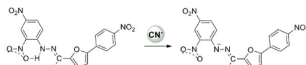
Fig. 9 A possible mechanism of L1 response to \text{CN}^- .
