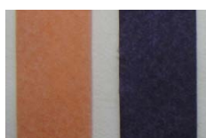
Fig. 7 Photographs of the L1 based test strips colorimetric detecting \text{CN}^- (from left to right: free test strip, test strip + \text{CN}^- ).
