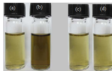
Fig.5 Optical photographs of the CuNCs prepared by the conventional method before (a) and after (b) added 0.5 ml of the Na 2 S solution (0.1M), and proposed method before (c) and after (d) added 0.5 ml of the Na 2 S solution (0.1M)
