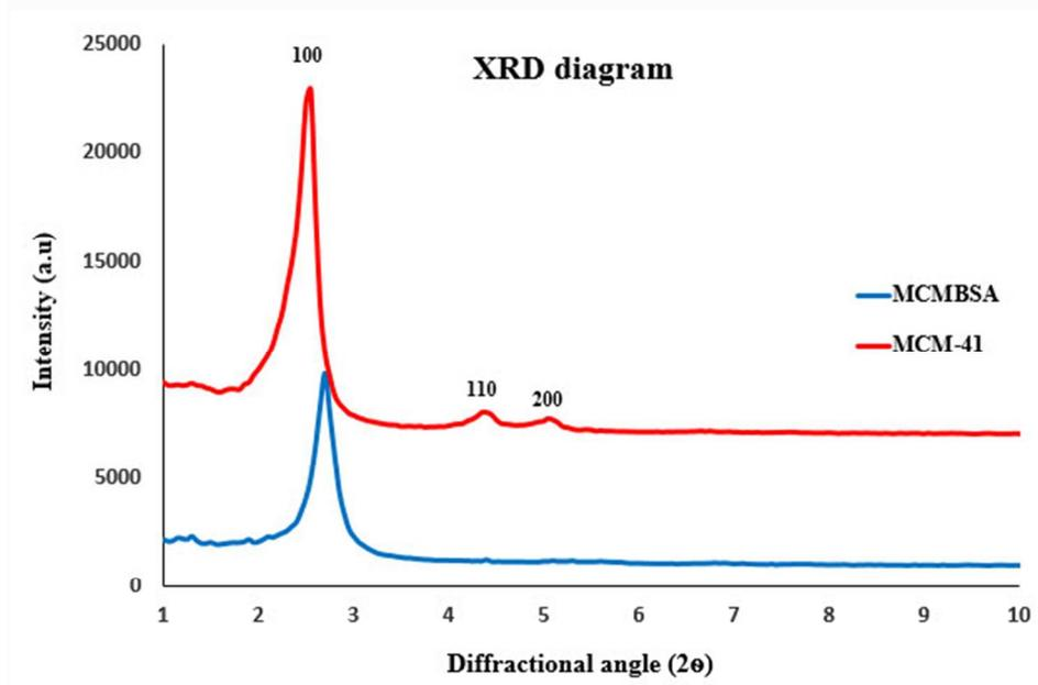
Figure 4 XRD patterns of MCM-41 and MCMBSA catalyst
