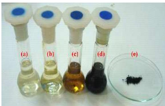
**Fig. 2.** Photograph of the reaction mixtures showing color change (a) Rosemary extract (b) Microemulsion including Pd ions (c) Stable colloid Pd nanoparticles prepared in W/O microemulsion (d) Reverse cylindrical AOT micelles including of Pd nanoparticles which pyrrole monomer polymerized along the surface of the reverse cylindrical micelles (e) Resulted PPy-Pd composite nanotubes.
