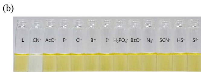
Figure 1. (a) Absorption spectral change of 1 (30 \mu M) in the presence of 70 equiv of various anions in a mixture of DMSO/bis-tris buffer (1:5, v/v). (b) Color change of receptor 1 (30 \mu M) in the presence of 70 equiv of various anions in a mixture of DMSO/bis-tris buffer (1:5, v/v).
