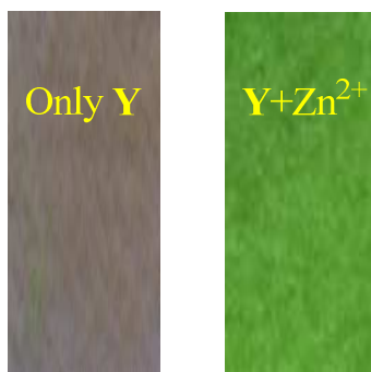
Fig. 6 Fluorescence change of the test strips of Y ( c=1 \times 10^{-3} M) with \text{Zn}^{2+} in DMSO/ \text{H}_2\text{O} ( v/v = 9/1 ) HEPES buffer solutions at \text{pH} = 7.2 under irradiation at 365 nm.
