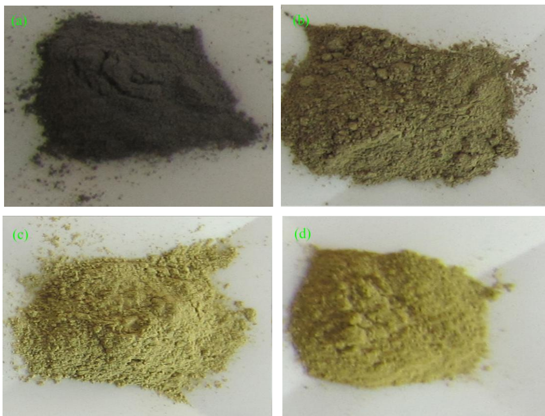
Fig. 1 Color of V_2O_5 - WO_3 / TiO_2 catalysts calcined in different atmosphere
