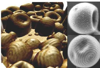
**Fig. 3** AFM and SEM images of block copolymer nanocapsules with corrosion inhibitors chemically encoded in the shell for a triggered release of both the corrosion inhibitor and a liquid self-healing agent present in the core of the nanocontainers.<sup>34</sup>
