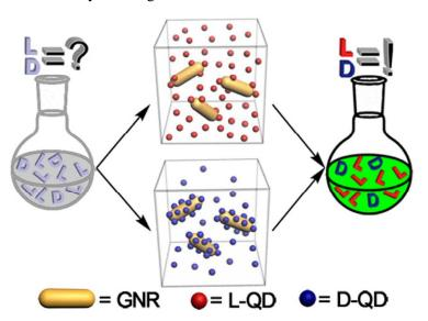
**Fig. 8.** Schematic illustration of nonexclusive QD/GNR based FRET sensors for chiral assays in two individual systems. Reproduced with permission from reference <sup>48</sup>.
