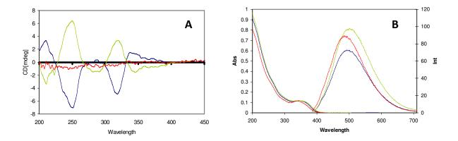
**Fig. 1**. **A**: CD spectra of D-Pen, (Red), L-Pen, (Green), and *Rac*-Pen, (Blue), modified CdS particles. **B**: UV-Vis (left) and emission spectra (right) of CdS nanocrystals stabilized with D-Pen (Blue), L-Pen (Green), and *Rac*-Pen (Red). Excitation wavelength for all emission spectra is 365nm. Reproduced with permission from reference <sup>3</sup>.
