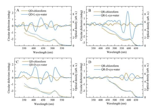
**Fig. 6.** Chiroptical properties of the CdSe/ZnS QD and QR solutions after chiral resolution. The absorption (dotted lines) and CD (solid lines) spectra of the chloroform and aqueous phases of the QDs (A and C) and QRs (B and D) after enantioselective phase transfer with L-cysteine (A and B) and D-cysteine (C and D). Reproduced with permission from reference <sup>21</sup>.
