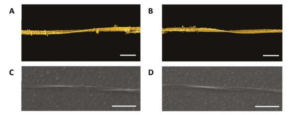
**Fig. 5**. Chirality of single CdTe nanoribbons. **A,B**, Surface rendering of the 3D TEM tomographic reconstruction of a LH (**C**) and a RH (**D**) nanoribbon. Scale bars, 100 nm. Reproduced with permission from reference <sup>20</sup>.
