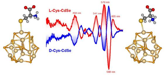
**Fig. 4**. Middle: CD spectra of L-Cys-CdSe (red curves) and D-Cys-CdSe (blue curves) and DFT optimized geometries of (left) L-Cys-(CdSe)<sub>13</sub> and (right) D-Cys-(CdSe)<sub>13</sub> NCs. Reproduced with permission from reference <sup>18</sup>.
