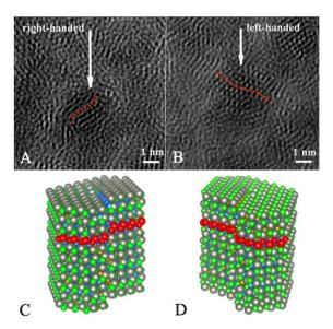
**Fig. 7.** (A, B) TEM images of the CdSe/ZnS QDs. The arrows indicate possible screw dislocations. (C, D) Atomistic models of CdSe/ZnS QDs with right (C) and left (D) screw dislocations. Dislocations are set in the (010) plane of CdSe core of nanocrystals with (-) Burgers vector (C) and (+) Burgers vector (D). Red dotted lines indicate the direction of the dislocations. Reproduced with permission from reference <sup>21</sup>.
