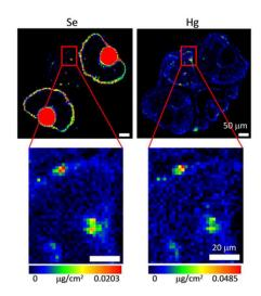
Fig. 5 Mercury selenium co-localization in zebrafish brain of fish exposed to 2  $\mu$ M HgCl<sub>2</sub>. The upper image of the entire section was imaged on APS 20-ID using a step size of 5  $\mu$ m and a dwell time of 0.6 s per pixel. The higher resolution image region (indicated with the red box) was collected subsequently using a step size of 2  $\mu$ m and a count time of 0.6 s per pixel.
