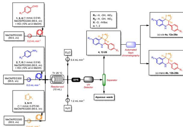
Fig. 3. Optimized flow set-up for the synthesis of the tricyclic tetrahydroquinoline library.
