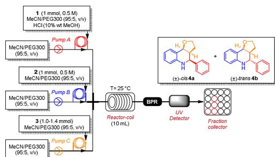
Fig. 2. General flow set-up employed during the reaction optimization.
