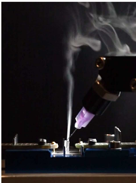
SAW-based fluid atomization device suitable for economic mass-scale production using a fluid supply via on-chip embedded SU-8 microchannels.
