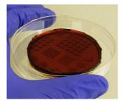
Leveraging techniques from the confectionary industry, we develop a candy-based process to fabricate microstructures in intrinsically soft silicone materials ( $E \approx 1$ kPa), and demonstrate the utility of this approach by developing a simple technique to measure forces generated by contractile microtissues.
