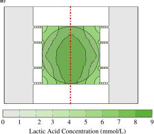
**Fig. 3** Glucose (a) and lactic acid (b) concentrations in picoliter bioreactor. The striped area indicates the position of the bacterial colony, while the dash dotted line shows plane of symmetry. The cells have been omitted from this picture.
