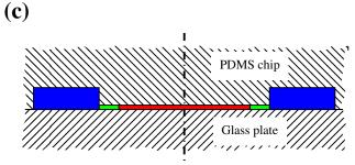
**Fig. A.1** Basic geometry of a lab-on-a-chip device. (a) shows a complete cell array, (b) a single chamber from above and (c) a side view with the position of PDMS chip and glass plate indicated. The dash dotted line shows the line of symmetry.
