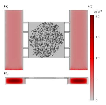
**Fig. 2** Velocity profiles: (a) Liquid velocity halfway between the bottom and the top of the chamber (b) Velocity profiles in the supply channels (c) Scale for velocities in m/s.
