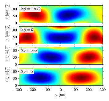
**Fig. 7** Color plots of the first-order pressure field for different values of phase difference  $\Delta \phi$ , as in Eq. (11), between the two incoming traveling waves. The position of the pressure node along the *y* direction can be tuned by changing the value of  $\Delta \phi$ . The pressure node moves by a distance of  $\lambda/8$  for each phase difference of  $\pi/2$ .
