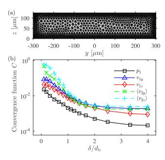
Fig. 3 Mesh convergence analysis. (a) An illustrative computational mesh with 2478 triangular elements obtained with maximum element size near the boundary,  $d_b = 30\delta$ , while the maximum element size in the bulk of the domain was set to  $20\,\mu\text{m}$ . (b) Semi-logarithmic plot of the relative convergence parameter C, as given in Eq. (21), for decreasing mesh element size near the boundaries,  $d_b$ .
