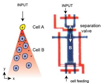
We present an automated microfluidic co-culture system that allows us studying the spatiotemporal signaling propagation from a single activated cell to a population of cells.
