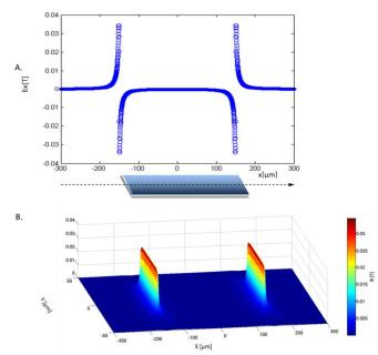
Fig. 4 The magnetic flux density (Bx) as simulated in MATLAB at 1  $\mu$ m above a ferromagnetic line, presented in 2D (A) and 3D (B).
