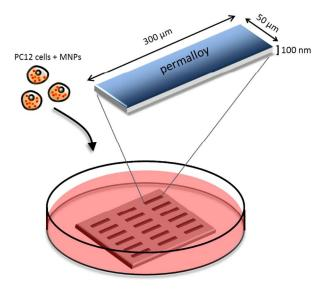
Fig. 3 An illustration describing the size of the permalloy patterns.
