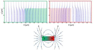
Fig. 5 The direction of the magnetic field at 1  $\mu$ m above the edges of a ferromagnetic line, as simulated in MATLAB.
