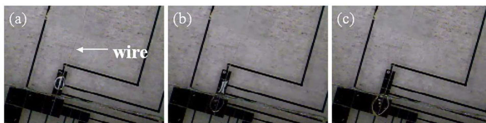
Fig. 10 Moving water drop across boundary from open to closed section. The voltage applied is 100 V_{\text{rms}} 100 Hz AC. Video 03 can be seen in the ESI.
