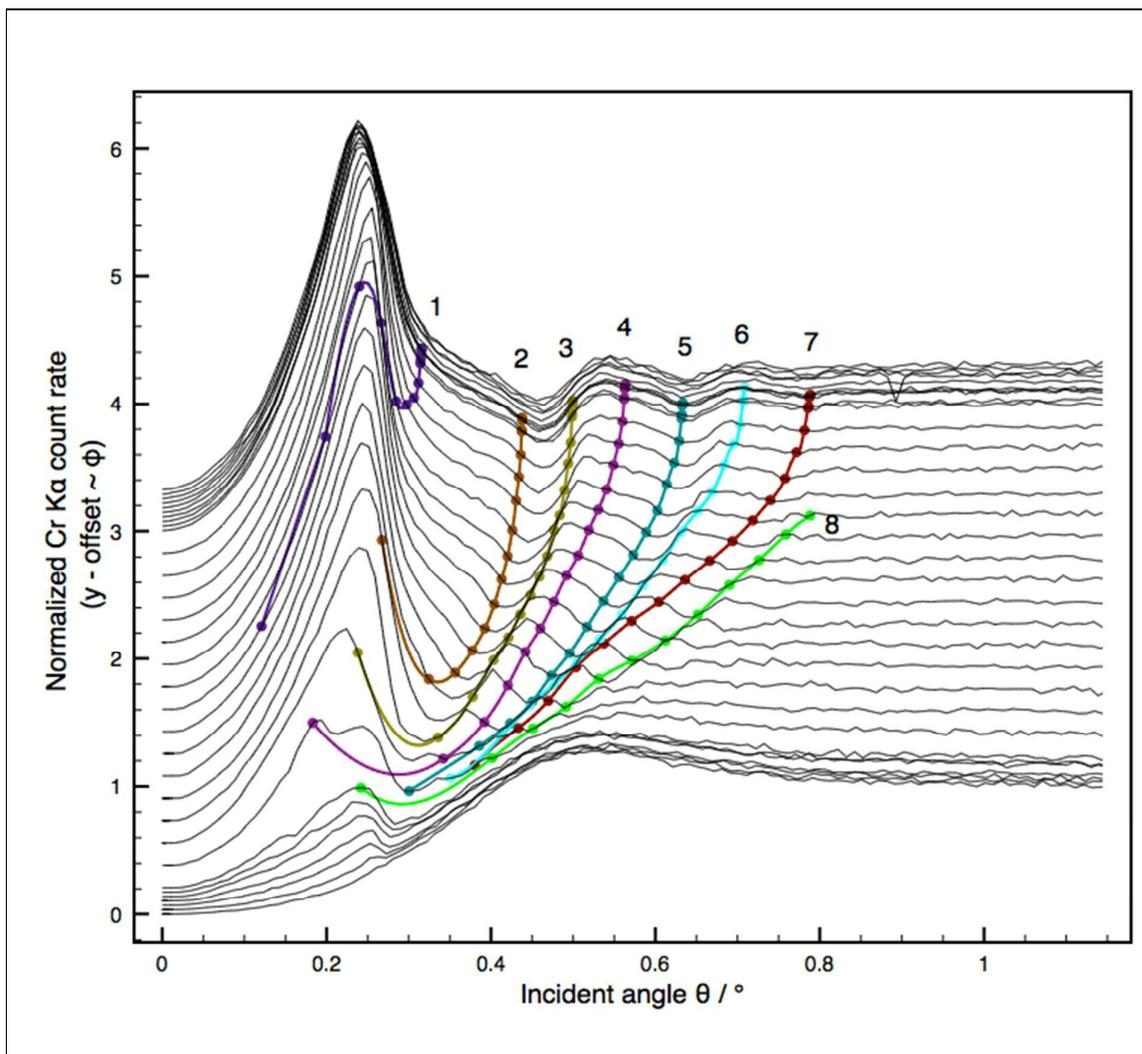
Fig. 1 Measured GIXRF profiles superposed with lines corresponding to  $M = 1, \dots, 8$ . The figure presents the same experimental data as presented in Figure 2 in the Comment [1].
