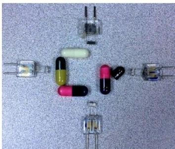
Trace levels of Cr in empty medicine capsules determined in less than 12 min sample<sup>-1</sup> (LOD = 0.4  $\mu\text{g g}^{-1}$ ).
