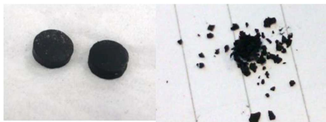
Figure 8. Photograph of SBR 8mm diameter disc samples before and after breakdown with G2 catalyst at room temperature over 24 h.
