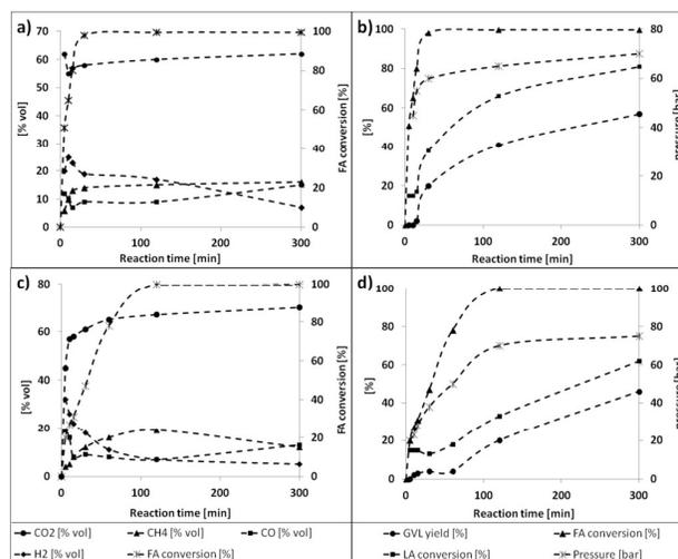
**Fig. 5** Product distribution as a function of reaction time for (a,b) Ru/C (Cl) HR and (c,d) Ru/C (Cl) LR.
