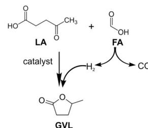
Scheme 1. GVL production from LA with FA as a hydrogen source
