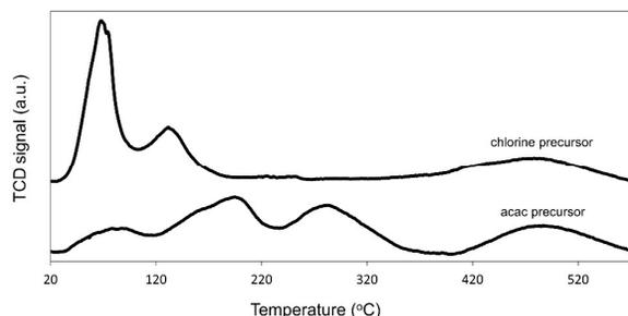
**Fig. 4** Temperature programmed reduction profiles of 5%Ru/C catalysts prepared from different precursors.
