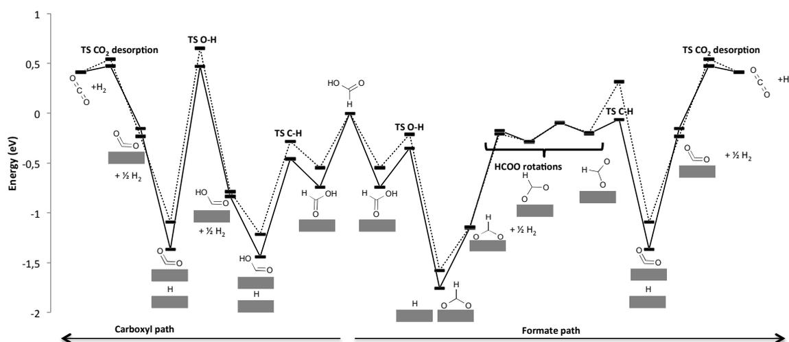
Fig. 6 Energy profile (in eV) for FA dehydrogenation on Ru (full line) and Cl-Ru (dashed line)- the reference is HCOOH in gas phase and bare slabs.
