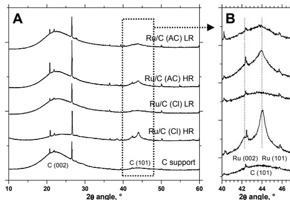
Fig. 1 Powder XRD pattern of Ru/C catalysts after reduction step at 200°C or 500°C, and of the bare high surface area carbon support. (A) Full diagram, (B) zoom on Ru (101) and Ru (002) diffraction peak zone, with overlap with the broad (101) peak of carbon.
