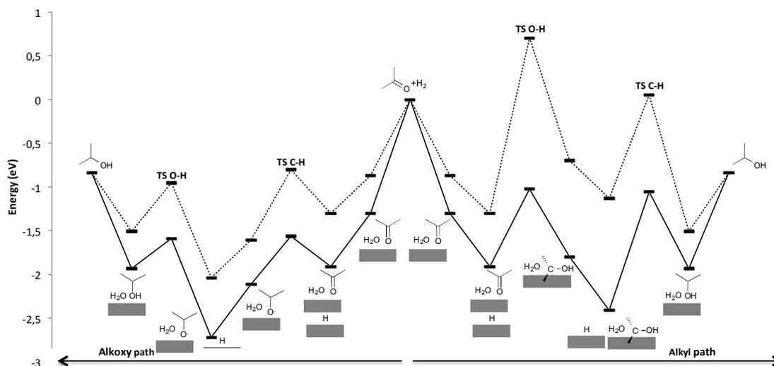
Fig. 7 Energy profile (in eV) for Acetone dehydrogenation on Ru (full line) and Cl-Ru (dashed line) - the reference is the acetone in gas phase, a H<sub>2</sub> molecule in gas phase, a bare slab and a hydrated slab with an H<sub>2</sub>O molecule adsorbed on it.
