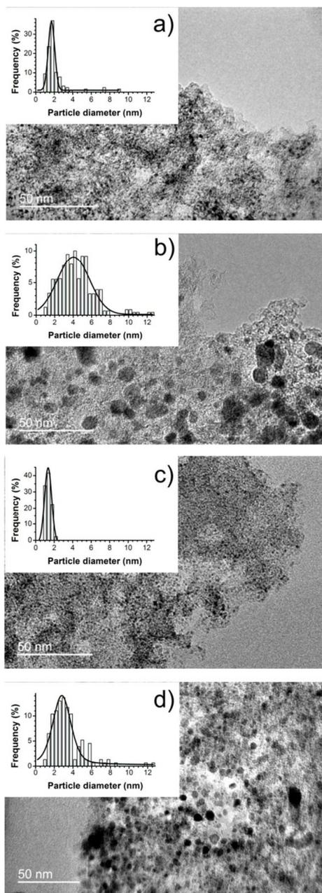
**Fig. 2.** TEM images and the corresponding metallic Ru nanoparticle size distribution histograms for Ru/C catalysts : (a) Ru/C (AC) LR, (b) Ru/C (AC) HR, (c) Ru/C (Cl) LR and (d) Ru/C (Cl) HR.
