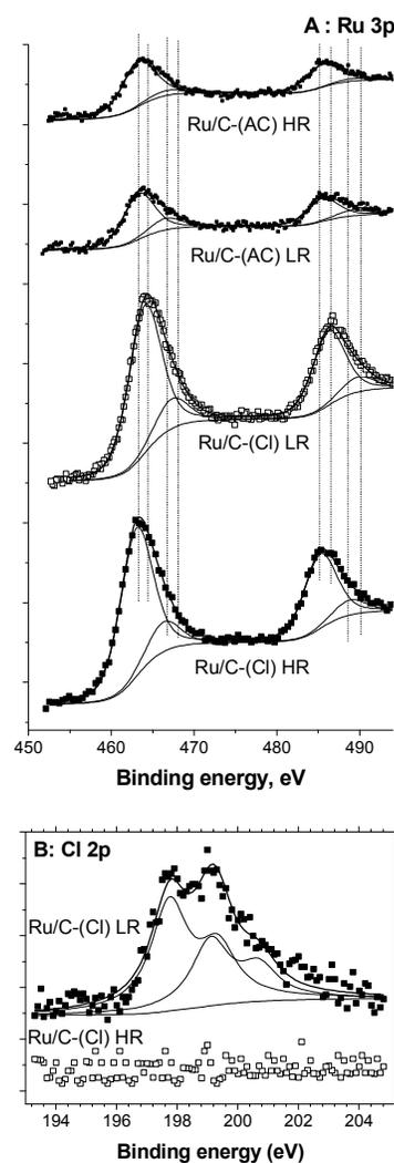
Fig. 3 (A) Ru  $3p$  and (B) Cl  $2p$  XPS spectra of the Ru/C catalysts.
