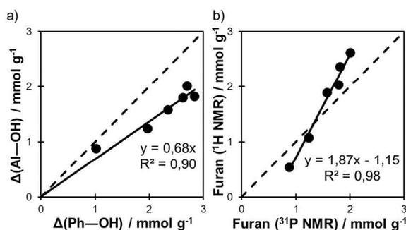
**Figure 2.** Correlation between the decrease in phenolic OH ( $\Delta(\text{Ph-OH})$ ) and the increase in aliphatic OH ( $\Delta(\text{AI-OH})$ ), as measured by  $^{31}\text{P}$  NMR (a), and correlation between the amount of linked furan groups as measured by  $^{31}\text{P}$  and  $^1\text{H}$  NMR (b).
