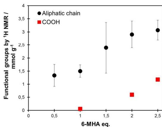
**Figure 7.** Functional groups calculated from  $^1\text{H}$  NMR. Spectra are available as supplementary information (Figure S6). The aliphatic chain has been calculated as the average of the integration regions 2.10 – 2.30 ppm (2H) and 1.00 – 1.80 ppm (6H).
