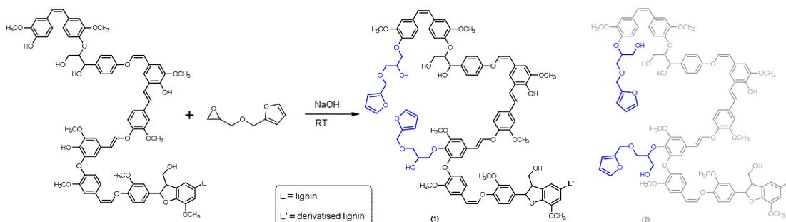
**Scheme 1.** Reaction of lignin with furfuryl glycidyl ether (FGE). (1) and (2) are the possible products.
