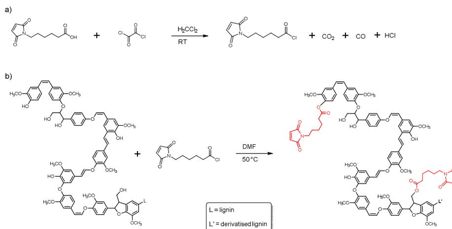
**Scheme 2.** 2-steps maleimidation of lignin: conversion of 6-maleimidoheptanoic acid (6-MHA) into the corresponding acyl chloride (a) and esterification of lignin with 6-maleimidoheptanoic acyl chloride (b).
