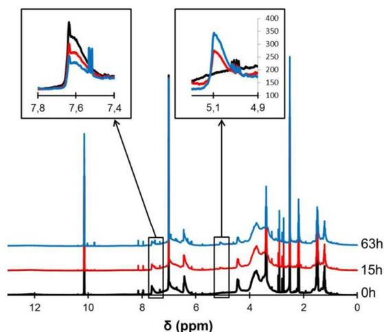
**Figure 10.**  $^1\text{H}$  NMR spectra of F50\_M50, measured after different time at 70 °C.
