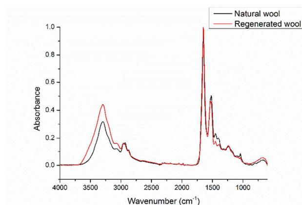
**Fig. 4** ATR-FTIR of natural wool and regenerated wool.
