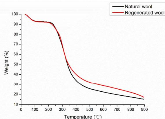
**Fig. 9** TGA plots of the natural wool and regenerated wool materials.
