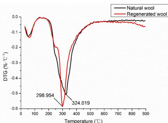
**Fig. 10** DTG plots of wool keratin fibres and regenerated wool keratin.
