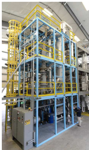
Pilot-scale catalytic biomass pyrolysis unit for producing low oxygen content, thermally stable bio-crude for upgrading into advanced biofuels.
