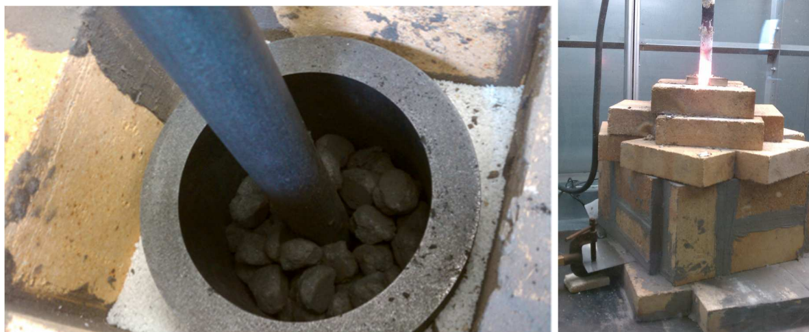
Figure 2a. Interior of the EAF with 1/3 of the feedstock loaded. b. EAF in operation, 50x50x100cm.
