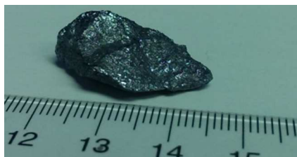
Figure 7. Typical broken silicon piece collected from EAF.
