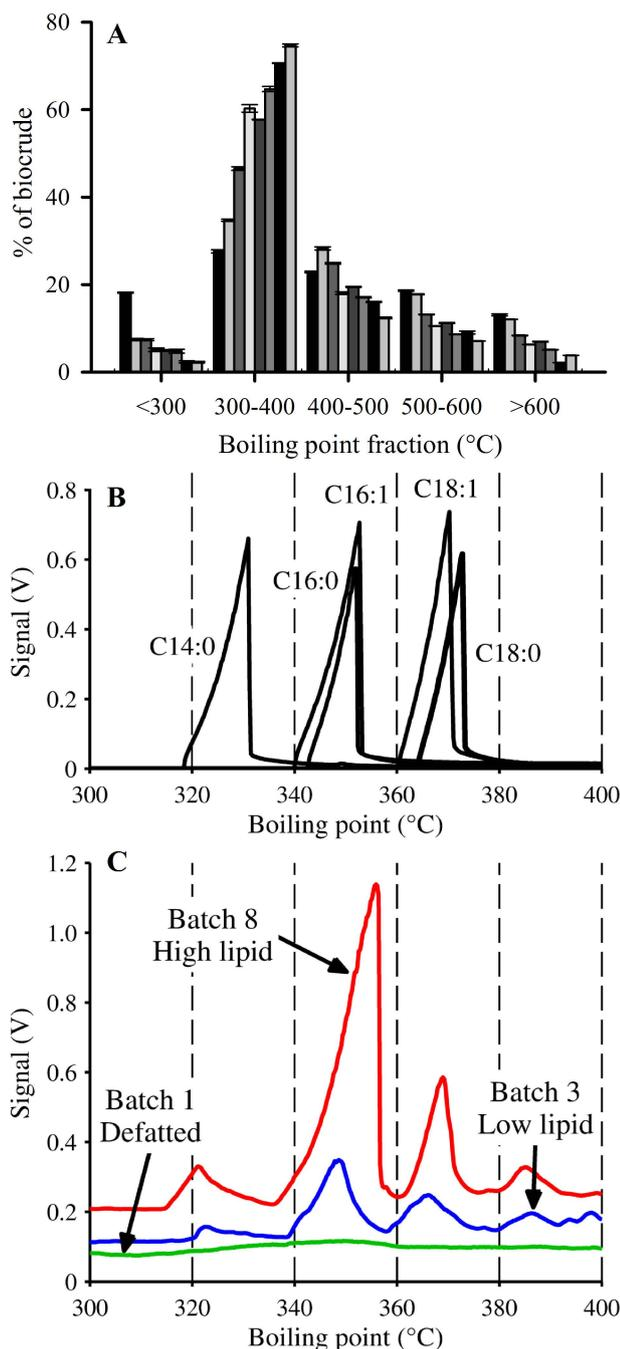
**Fig 4** A) Biocrude product boiling point (BP) distribution via SimDist analysis. Bars are ordered in increasing lipid content (Batch 1 to 8) from left to right. B) BP profile within 300–400 °C of individual fatty acids for reference to (C). C) BP profile within 300–400 °C of biocrudes derived from HTL of three representative batches of *Nannochloropsis*.
