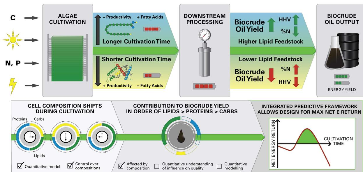
**Fig. 1** The integrated modeling framework allows for prediction and optimization of system-scale parameters for the microalgae-HTL biofuel system. The top half of the figure represents the integrated processing scheme for microalgae HTL, with the black arrows representing decisions on cultivation times that lead to downstream implications. The bottom half represents the current research progress towards formulating an integrated predictive framework.
