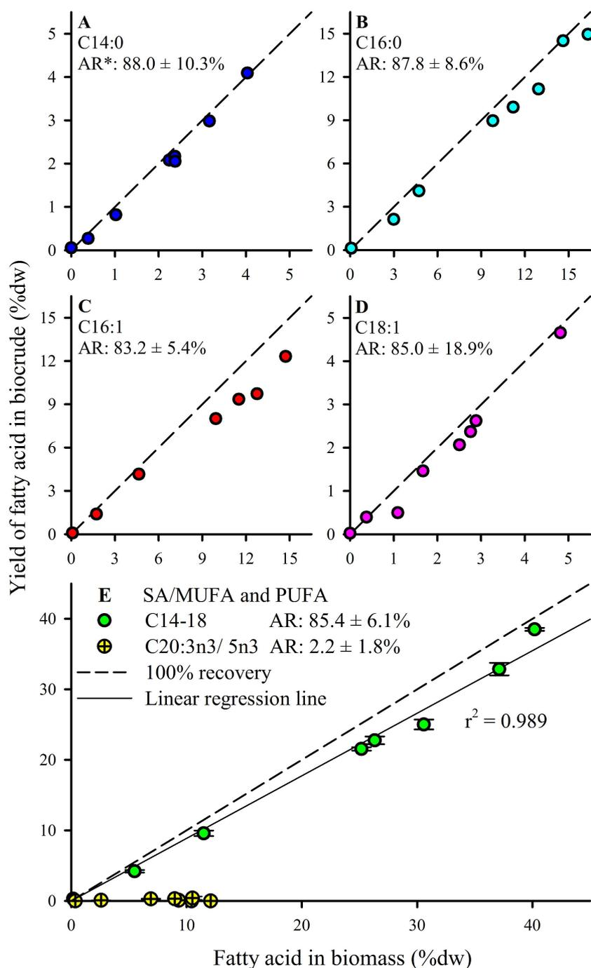
**Fig. 5** Biocrude product fatty acid (FA) analysis reported as %dw yield for FAs with >1%dw yield observed. \* Average recovery, computed using all batches except the defatted batch. Diagonal dashed line indicates 100% recovery of feedstock FA in the biocrude product. Error bars in panel E indicates min/max values from replicate analysis; error bars for individual FAs in panels A-D were smaller than the size of the symbols shown.
