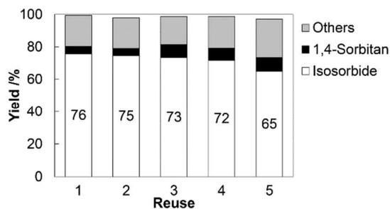
**Fig. 2** Reuse experiments of H $\beta$ (75) in the dehydration of sorbitol at 400 K for 2 h.
