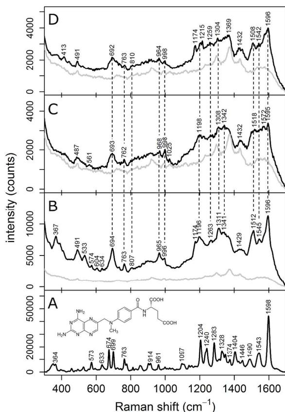
Figure 1 (A) Normal Raman spectrum of MTX powder; (B) SERS spectrum of MTX 10  $\mu\text{M}$  in PBS, (C) SERS spectrum of MTX in 4% BSA-PBS, and (D) SERS spectrum of MTX diluted in human serum (1:4, v/v). The background signal of the substrate (grey line) is reported for comparison together with SERS spectra. The chemical structure of MTX is reported for reference in (A). All spectra were collected using an excitation at 785 nm.
