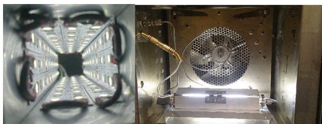
Figure 4. LED light configuration. Left, detail of the inner LED distribution. Right, microreactor in the oven surrounded by the LEDs.
