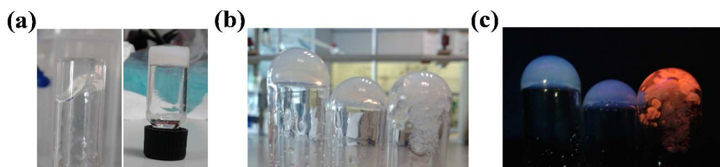
Figure 8. (a) Ligand hydrogels formed of 2\cdot(S,S) at 6 wt% (left) and 10 wt%. (b) Ligand hydrogels formed at 6 wt% (left), 10 wt% (middle) and Eu(III)-doped 5 wt% hydrogel, under ambient light (c) under UV light ( \lambda = 254 nm).
