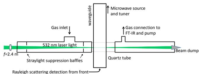
**Fig. 2** Schematic of the microwave plasma source used for CO<sub>2</sub> dissociation. Indicated is the laser beam path that is used for Rayleigh scattering experiment.
