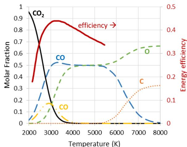
**Fig. 9** Chemical Equilibrium calculated molar fraction of the products of CO<sub>2</sub> dissociation at a fixed pressure of 100 mbar. Calculated energy efficiencies assuming instantaneous quenching after Polak *et al.* are plotted on the right axis.
