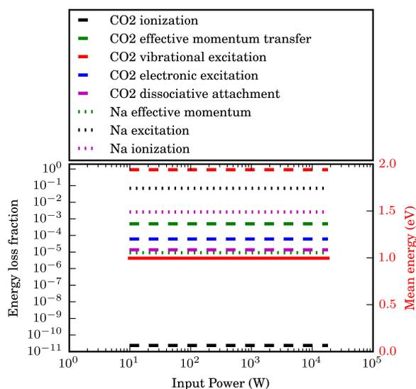
**Fig. 11** The effect of 0.01% sodium added to a CO<sub>2</sub> microwave discharge on the relative energy loss fractions for the main processes at play. It shows that vibrational excitation has become the dominant energy loss channel for the electrons, which does not change within the conditions as investigated in the present work.
