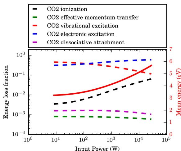
**Fig. 8** Energy loss fractions for the various processes at play in a CO<sub>2</sub> microwave discharge. It shows that vibrational excitation is not the dominant energy loss channel for the electrons in conditions as investigated in the present work.
