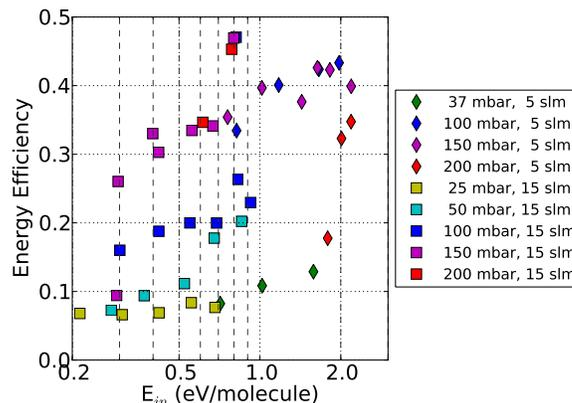
**Fig. 5** Energy efficiency measured in pure microwave CO<sub>2</sub> plasma as a function of the specific energy input, at 5 and 15 slm gas flow rate, in scans of the reactor pressure. The underlying experimental data are identical to those of Figure 4.
