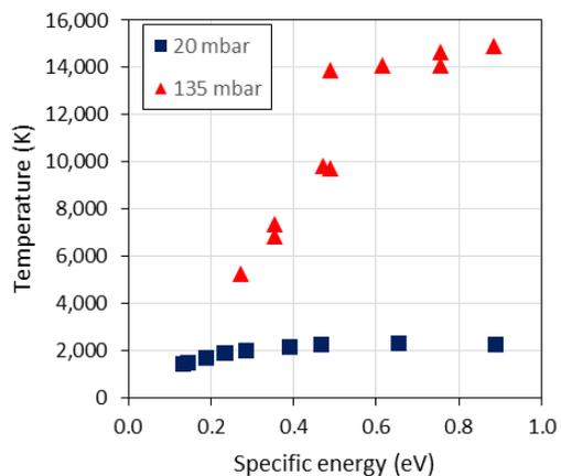
**Fig. 6** Gas temperatures determined from neutral gas density measurements with Rayleigh scattering and reactor pressure readings in a scan of specific energy input. The gas flow was at 13 slm similar to the high flow conditions in Figure 4 and 5, the pressure was tuned to 20 and 135 mbar, respectively.
