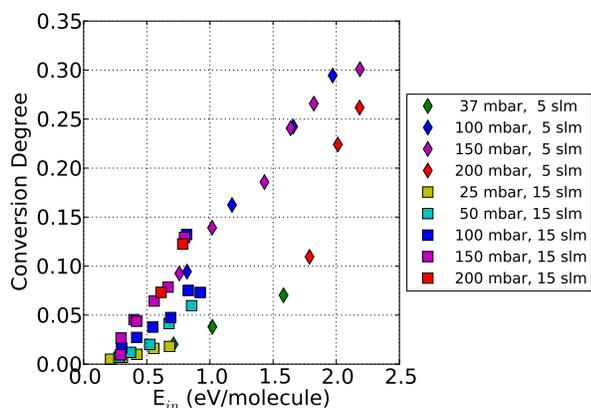
**Fig. 4** Conversion degree measured in pure microwave CO<sub>2</sub> plasma as a function of the specific energy input, at 5 and 15 slm gas flow rate, in scans of the reactor pressure.
