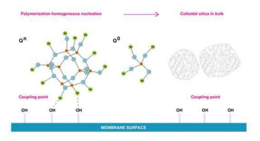
Figure 12 - Dissolved silica polymerisation in CP layer on the membrane surface in medium and high salinity waters without presence of aluminium.
