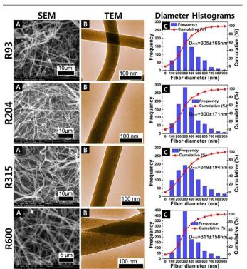
Figure 5. SEM (A), TEM (B) and fibre diameter distributions (C) of  $Al_2O_3$  fibres calcined at 650°C for 4 hr R93(93°C/hr), R204(204°C/hr),R316(316°C/hr), and R600(600°C/hr).
