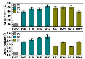
Figure 10. Al Content(Top) and Density of Alumina fibre(Bottom) (A)PVP01, (B)S650-S950, and (C)R93-R600.
