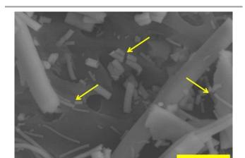
Figure 11. Scanning electron micrograph of alumina fibre S950(950°C) illustrating transverse fibre breakage (see arrows) after exposure to PSF for 28 days.  $Scalebar = 1 \mu m$ .
