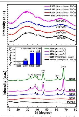
Figure 6. XRD Patterns and crystallinity of  $Al_2O_3$  fibres calcined at different soak temperatures and ramp rates.
