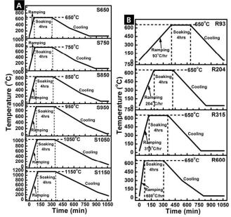
Figure 2. Temperature profiles of the variations in the heating cycles to calcine the alumina precursor – PVP fibres to fabricate the  $Al_2O_3$  fibres. (A) Variation in soak temperatures (samples labelled S650 to S1150). (B) Variation in heating ramp rates (samples labelled R93, R204, R315, and R600)
