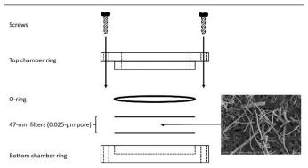
Figure 3. Static dissolution chamber assembly; SEM micrograph of S950 material after 7 day exposure to SUF
