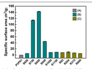
Figure 8. Specific surface area of Alumina fibres. (A) PVP01, (B) fibres rapidly heated to final soak temperatures (S650-S1150); (C) fibres heated at different ramp rates to soak temperature 650°C(R93- R600).
