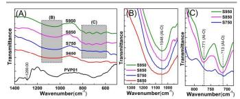
Figure 7. FT-IR spectra of precalcined polymer PVP composite (PVP01) and the calcined  $Al_2O_3$  fibres at various soak temperatures (S650 – S950).
