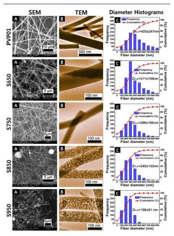
Figure 4. SEM (A), TEM (B) and length weighted frequency distribution of fibre size; (C) of the uncalcined fibres and the fibres calcined for 4 hr at different temperatures.
