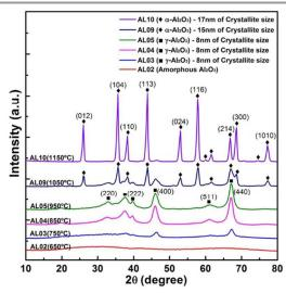
Figure 9. XRD Plots of alumina fibres calcined at 650 - 1150 °C.
