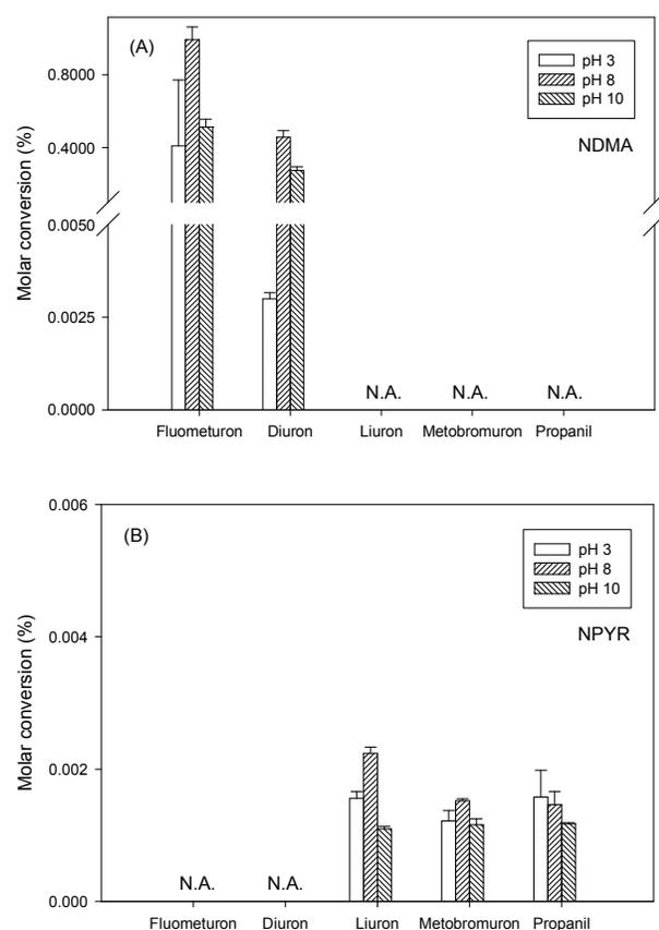
Figure 5. (A) NDMA and (B) NPYR molar conversions during dichloramination of phenylurea herbicides at pH  $8 \pm 0.2$  for a contact time of 24 hours. The initial concentrations of herbicides, ammonia, and disinfectants were  $9 \mu\text{M}$ ,  $0.12 \text{ mM}$ , and  $0.1 \text{ mM}$ , respectively. The error bars depict one standard deviation. N.A. (non-available) indicates that the experiments were not conducted.
