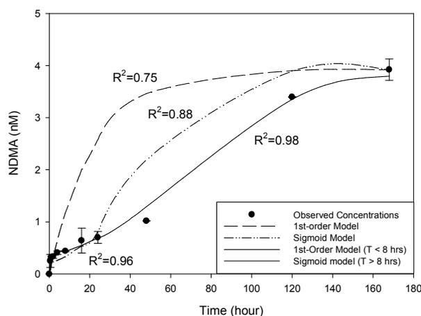
Figure 2. Observed and simulated kinetics of NDMA formation from fluometuron upon monochloramine disinfection (Error bars represent the 95% confidence level). The initial concentrations of fluometuron and  $\text{NH}_2\text{Cl}$  were 9  $\mu\text{M}$  and 0.1 mM, respectively. The pH was at  $\text{pH } 8 \pm 0.2$ .
