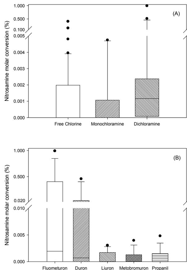
Figure 6. Nitrosamine molar conversions observed in all experiments using (A) different disinfectants (the free chlorine data includes those from the experiments with additional nitrogen sources) and (B) different phenylurea herbicides. The contact time
