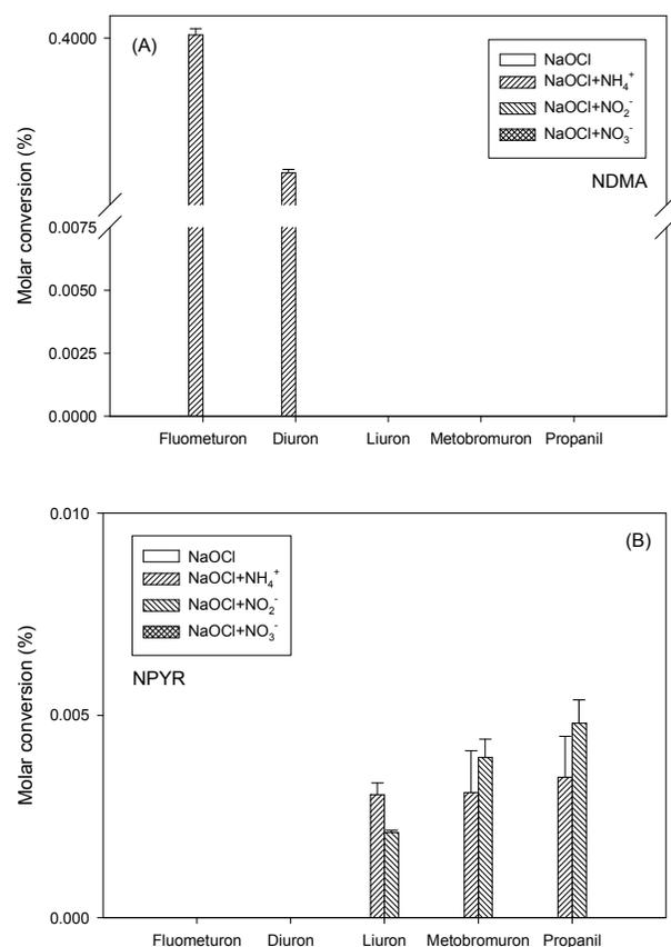
Figure 4. (A) NDMA and (B) NPYR molar conversions during chlorination of different phenylurea herbicides with/without the presence of additional nitrogen sources at pH  $8 \pm 0.2$  for a contact time of 24 hours. The initial concentrations of herbicides, nitrogen, and disinfectants were  $9 \mu\text{M}$ ,  $0.12 \text{ mM}$ , and  $0.1 \text{ mM}$ , respectively. The error bars depict one standard deviation. Blanks indicate that nitrosamine formation was non-detected.
