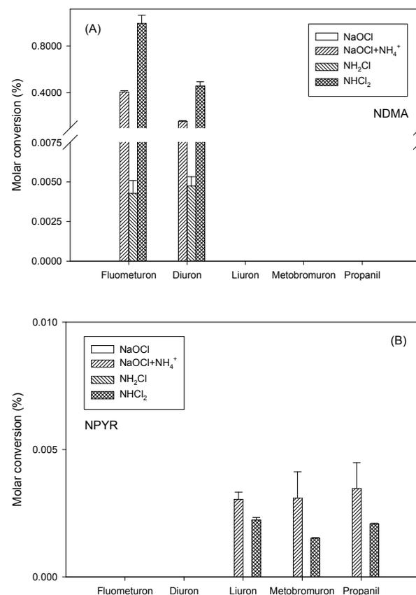
Figure 3. (A) NDMA and (B) NPYR molar conversions from different phenylurea herbicides under different disinfection scenarios at pH  $8 \pm 0.2$  for a contact time of 24 hours. The initial concentrations of herbicides,  $\text{NH}_4^+$ , and disinfectants were  $9 \mu\text{M}$ ,  $0.12 \text{ mM}$ , and  $0.1 \text{ mM}$ , respectively. The error bars depict one standard deviation. Blanks indicate that nitrosamine formation was non-detected.
