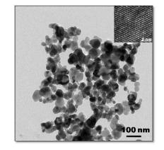
Figure 1: TEM image of  $La_2O_3$  NP. The particles are irregular spheres in shape and less than 100 nm. Inset shows the lattice spacing (0.348 nm).
