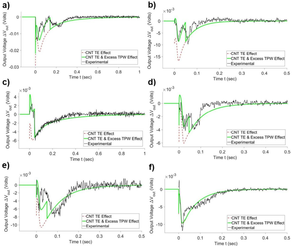
Figure 4 a-f) Thermopower wave voltage output prediction for experimental samples. The experimental output is shown in black, the model-predicted thermoelectric output is shown in red dotted lines, and the final model-predicted output is shown in green.
