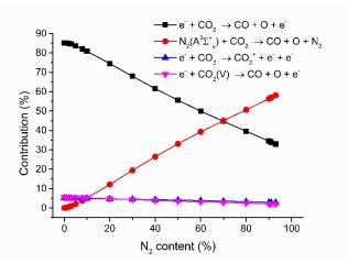
Figure 5: Relative contribution of the main processes leading to  $CO_2$  conversion as a function of  $N_2$  content, for a residence time of 0.73 s and a SEI of approx. 12 J  $\rm cm^{-3}$ .
