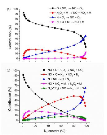
Figure 6. Relative contributions of the main formation (a) and loss (b) mechanisms of NO as a function of  $N_2$  content, for a residence time of 0.73 s and a SEI of approx. 12 J cm<sup>-3</sup>.
