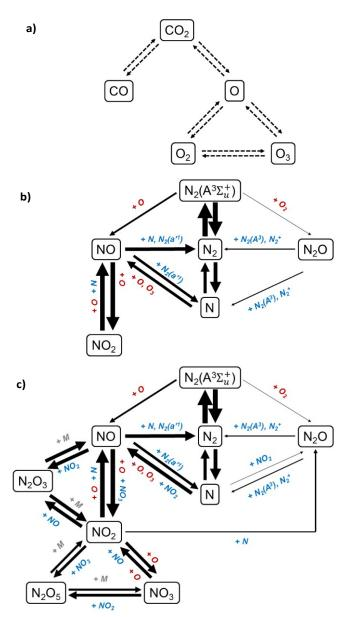
Figure 9. Reaction scheme to illustrate the main pathways of the  $N_2O$  and  $NO_\chi$  chemistry as predicted by the model. Reaction paths starting from  $CO_2$  (a), initiation of the  $NO_\chi$  chemistry (b), complete overview of the  $N_2O$  and  $NO_\chi$  chemistry (c). The thickness of the arrows corresponds to the importance of the reactions.
