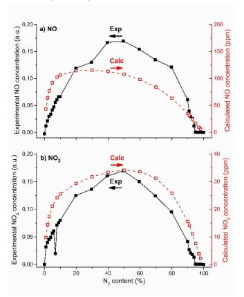
Figure 2. Experimental and calculated concentrations of NO (a) and NO  $_2$  (b) as a function of  $N_2$  content, for a residence time of 0.73 s and a SEI of approx. 12 J cm  $^{\circ}$
