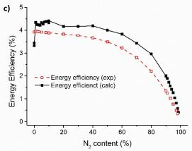
Figure 1. Experimental and calculated values of absolute  $CO_2$  and  $N_2$  conversion (a), effective  $CO_2$  and  $N_2$  conversion (b) and energy efficiency of  $CO_2$  conversion (c) as a function of  $N_2$  content, for a residence time of 0.73 s and a SEI of approx. 12 J cm<sup>-3</sup>.
