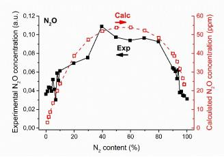
Figure 4. Experimental and calculated concentrations of  $N_2O$  as a function of  $N_2$  content, for a residence time of 0.73 s and a SEI of approx. 12 J cm<sup>-3</sup>.
