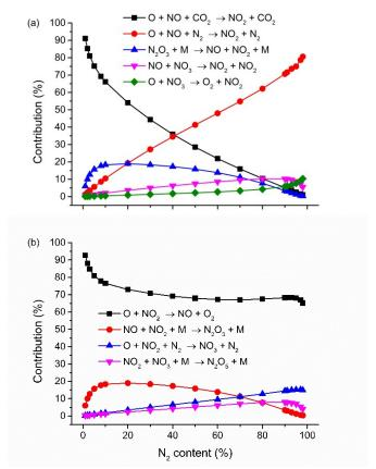
Figure 7. Relative contributions of the main formation (a) and loss (b) mechanisms of  $NO_2$  as a function of  $N_2$  content, for a residence time of 0.73 s and a SEI of approx. 12 J cm<sup>-3</sup>.
