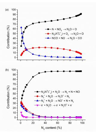
Figure 8. Relative contributions of the main formation (a) and loss (b) mechanisms of  $N_2O$  as a function of  $N_2$  content, for a residence time of 0.73 s and a SEI of approx. 12 J cm<sup>-3</sup>.
