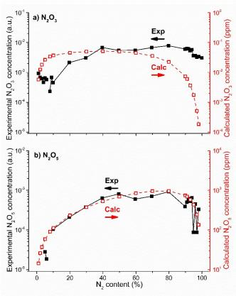
Figure 3. Experimental and calculated concentrations of  $N_2O_3$  (a) and  $N_2O_5$  (b) as a function of  $N_2$  content, for a residence time of 0.73 s and a SEi of approx. 12 J cm
