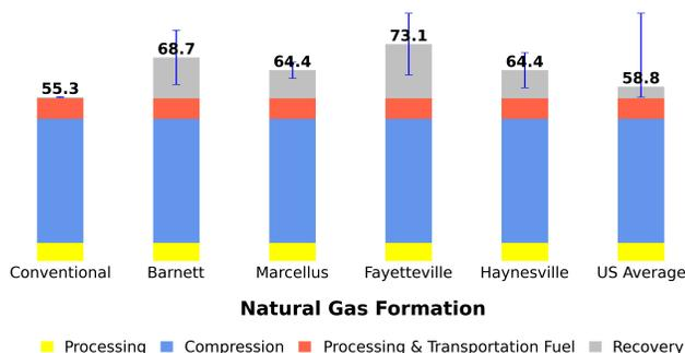
Fig. 7 Life cycle water consumption (L/GJ) of CNG derived from different formations.
