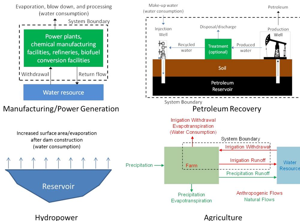
**Fig. 1** Definitions of water consumption. Upper left: Flows of water into and out of manufacturing facilities and power plants. Upper right: Flows of water and petroleum in recovery operations. Lower left: Increased evaporation from construction of hydropower facilities. Lower right: Natural and anthropogenic flows of water on an agricultural land segments.
