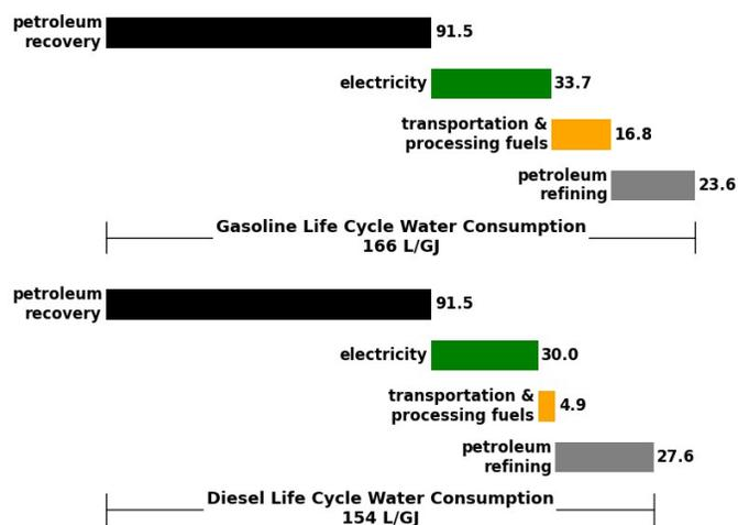
Fig. 4 Petroleum gasoline and diesel life cycle water consumption breakdown.
