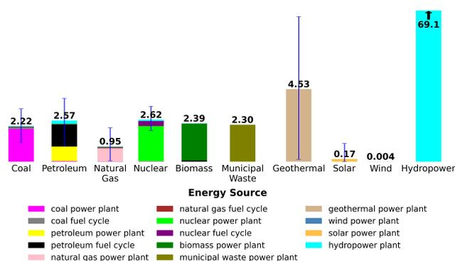
Fig. 8 Life cycle water consumption (L/kWh) associated with electric power generation facilities.
