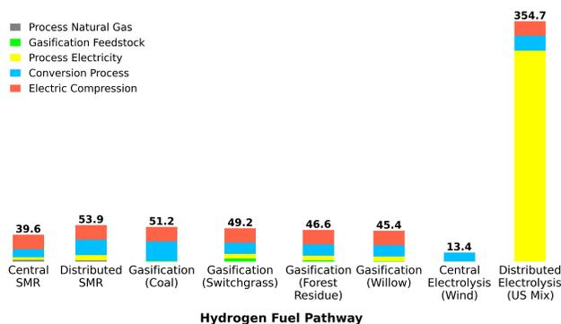
**Fig. 10** Life cycle water consumption (L/kg H<sub>2</sub>) associated with compressed H<sub>2</sub> fuel generation pathways.
