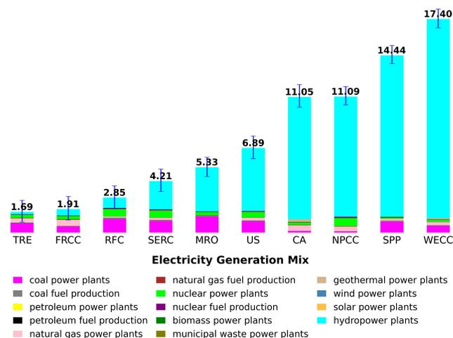
**Fig. 9** Life cycle water consumption (L/kWh) from various US electricity generation mixes.
