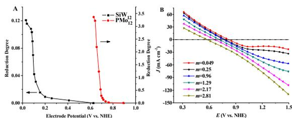
Fig. 5 (A) Electrode potential (25 °C) of  $\text{PMO}_{12}$  and  $\text{SiW}_{12}$  ( $0.3 \text{ mol l}^{-1}$ ) on graphite at different value of  $m$ . Pt wire was used as counter electrode and a saturated calomel electrode (SCE) was used as reference electrode. (B) Linear potential sweep curves of  $\text{PMO}_{12}$  ( $0.3 \text{ mol l}^{-1}$ )-glucose solution (25 °C) at different reduction degree in a three electrode compartment using a polished graphite rod as working electrode.
