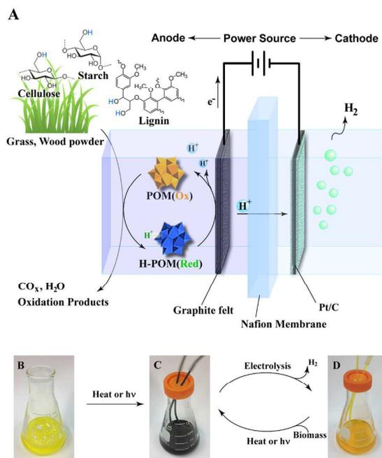
**Fig. 1** (A) Schematic illustration of the chemical-electric conversion process. Anode is a simple graphite-felt electrode; cathode is a gas-diffusion electrode loaded with Pt black catalyst ( $4 \text{ mg cm}^{-2}$ ). (B) Solution of POM-biomass before heating or light irradiation. (C) The colour change of biomass-POM mixture after heating. (D) The biomass-POM solution after electrolysis for hydrogen production.
