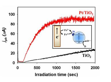
Fig. 3. Comparison of  $Fe^{3+}$ -mediated photocurrents collected on a Pt electrode for TiO<sub>2</sub> and Pt/TiO<sub>2</sub>. The inset shows the current collection on an inert Pt electrode immersed in UV-illuminated Pt/TiO<sub>2</sub> suspension. Adapted with permission from Ref. 150 (Copyright 200 2014 American Chemical Society).
