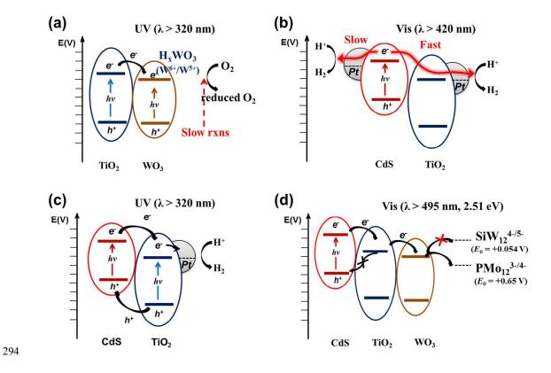
Fig. 10. Schematic illustration of the electron-transfer processes in multi-junction systems under UV and visible light. (a) TiO<sub>2</sub>/WO<sub>3</sub>, (b, c) CdS/TiO<sub>2</sub>/Pt, and (d) CdS/TiO<sub>2</sub>/WO<sub>3</sub>.
