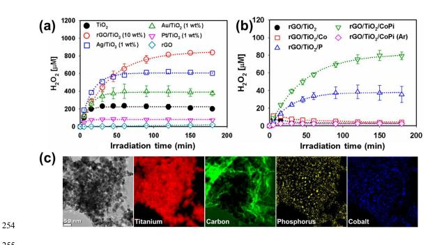
Fig. 7. Photocatalytic production of  $H_2O_2$  (a) in the presence of 2-propanol and (b) in the absence of 2-propanol as a result of water oxidation. (c) TEM image and EELS mapping of rGO/TiO<sub>2</sub>/CoPi. Reproduced from Ref. 151 with permission from The Royal Society of Chemistry.
