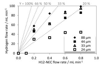
Fig. 4 – Dehydrogenation of H12-NEC – effect of H12-NEC flow variation on hydrogen yields: Reaction temperature: 260 °C; catalyst: 24 μm, 33 μm, 44 μm, 88 μm; 30 catalyst spheres; <sup>35</sup> platinum mass between 0.36-1.87 mg.
