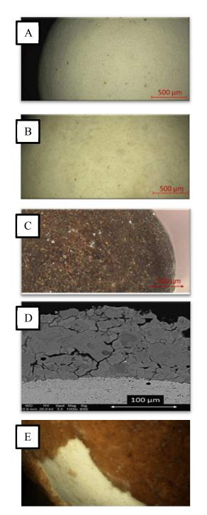
Fig. 2 - Sphere coating: Top down: (A) – Uncoated; (B) – Coated; (C) – Impregnated; (D) – Coating layer; (E) – Impregnated coating, partially removed.
