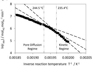
Fig. 9 – Arrhenius plot for the 24  $\mu$ m catalyst: Reaction temperature: 224 °C – 261 °C; H12-NEC flow rate 0.6 mL min<sup>-1</sup>; active layer of catalyst: 24  $\mu$ m; 30 catalyst spheres; Pt mass <sup>40</sup> 0.36 mg; H<sub>2</sub>-yield < 33 %; constant slopes (kinetic vs. pore diffusion regime) are displayed as dashed lines.
