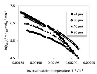
**Fig. 8** – Arrhenius plot derived from all experimental data <sup>10</sup> obtained in this study: Reaction temperatures: 224 °C - 261 °C; H12-NEC flow rate 0.6 mL min<sup>-1</sup>.
