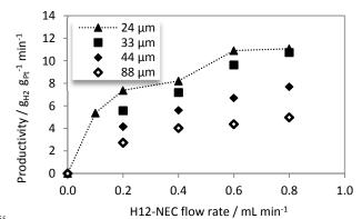
**Fig. 5** - Catalyst productivity as function of H12-NEC flow rate: Reaction temperature: 260 °C  $\pm$  1 °C; catalysts: 24 µm, 33 µm, 44 µm, 88 µm; 30 catalyst spheres; Pt mass in reactor: 0.36-1.87 mg; productivity defined as gram H<sub>2</sub> released per gram Pt.
