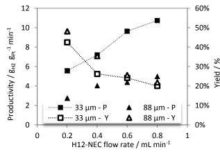
**Fig. 6** – Productivity and corresponding yield: Reaction <sup>50</sup> temperature: 260 °C  $\pm$  1 °C; catalysts: 33 µm, 88 µm; 30 catalyst spheres; Pt mass: 0.82 mg and 1.87 mg.
