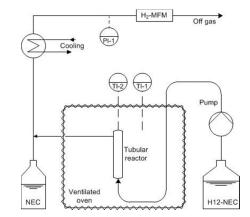
Fig. 1 - Continuous dehydrogenation setup schematic
