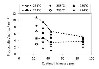
Fig. 7 – Productivity as a function of diffusion length: Reaction 70 temperature: 224 °C – 261 °C; H12-NEC flow rate 0.6 mL min<sup>-1</sup>; catalysts: 24  $\mu$ m, 33  $\mu$ m, 44  $\mu$ m, 88  $\mu$ m; 30 catalyst spheres; Pt mass: 0.36-1.87 mg.
