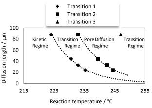
**Fig. 11** – Reaction regime map: Reaction temperature: 224 °C – 261 °C; H12-NEC flow rate 0.6 mL min<sup>-1</sup>; Catalysts: 24 μm, 33 μm, 44 μm, 88 μm; 30 catalyst spheres; Platinum mass: 0.36-
