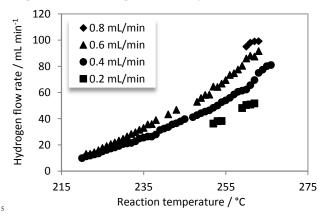
Fig. 3 - Dehydrogenation of H12-NEC as a function of temperature: Reaction temperature between 220 °C and 266 °C; H12-NEC flow rates between 0.2 mL min<sup>-1</sup> and 0.8 mL min<sup>-1</sup>; catalyst spheres with 33  $\mu$ m coating thickness; 30 spheres applied <sup>10</sup>  $\cong$  0.82 mg of total Pt.
