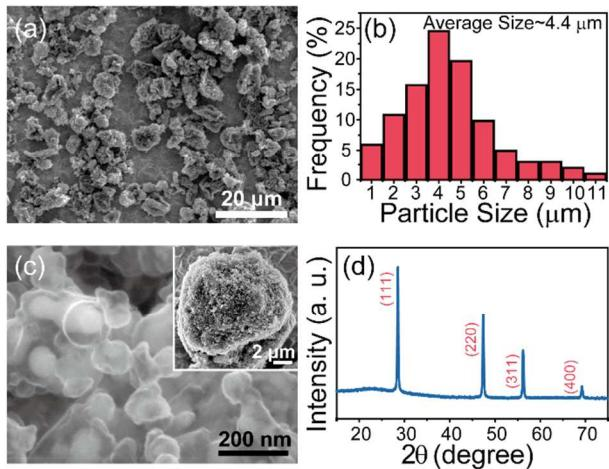
**Figure 2. Characterization of nano-Si SC** (a) Low-magnification SEM image showing the size distribution of SC. (b) Statistical analysis of the distribution of SCs' size based on (a). (c) Magnified SEM image of the surface of SC showing the well-defined void space as well as intact carbon framework. Inset image shows one typical cluster. (d) X-ray diffraction pattern of as-obtained nano-Si SC powders.
