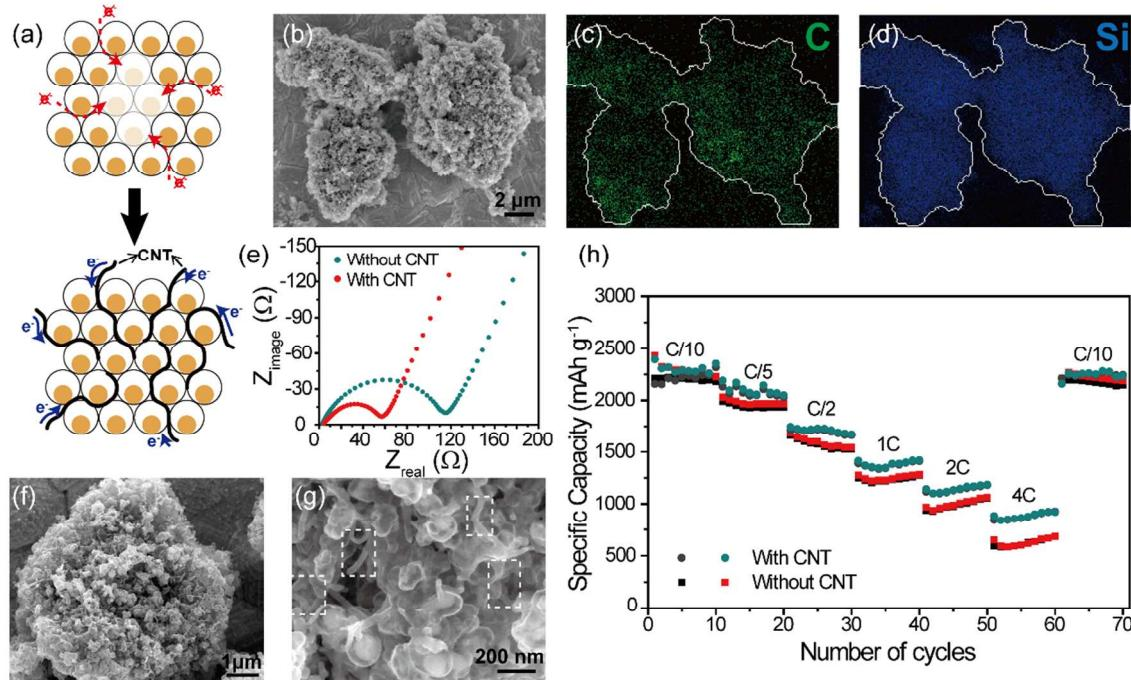
**Figure 4. CNT-embedded Nano-Si SC for improved intracluster conductivity.**
