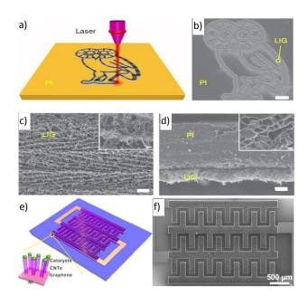
Figure 11. a)-d) Laser-induced graphene formed from commercial PI films using a  $CO_2$  laser under ambient conditions. Copyright (2014) Nature Publishing Group. e) and f) Schematic and SEM images of the G/CNTCs based microsupercapacitor. Reprinted with permission.<sup>107, 108</sup>
