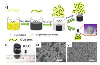
Figure 13. a) Illustration of the formation of HDGS and LDGS. b) Optical photos of LDGS and HDGS. SEM images of (c) LDGS and (d) HDGS. Reprinted with permission.<sup>116</sup>
