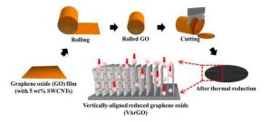
Figure 5. Schematic illustration of the fabrication of vertically aligned rGO. Reprinted with permission.<sup>72</sup>
