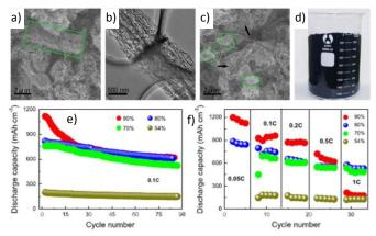
Figure 12. a) SEM and b) TEM of the pristine aligned CNTs. c) SEM and d) photograph of the aligned CNT/S composite. e) and f) cycle performance and rate performance of the aligned CNT/S composite with different sulfur content. Reprinted with permission.<sup>112</sup>
