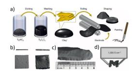
Figure 9. Schematic of MXene clay synthesis and electrode preparation. a) The fabrication and preparation process of MXene. b) Shrinking (left) and swelling (right) of MXene. c) Image of a rolled film and d) Shaped MXene into letter M with high conductivity. Reprinted with permission.<sup>96</sup>
