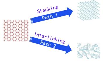
Figure 3. Two typical extreme models of the assembly of graphene or functionalized graphene sheets into other carbon architectures
