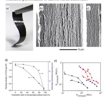
Figure 4. Characterization of a liquid electrolyte-mediated chemically converted graphene film (CCG). a) Photograph of the flexible film. b) and c) SEM images of the cross section of the CCG film with different contents of liquid electrolyte (78.9 27.2 vol % of  $H_2SO_4$ ). d) Relationship between the packing density and the interlayer spacing versus  $H_2SO_4$  content. e) Ragone plot of the film. Reprinted with permission.<sup>46</sup>
