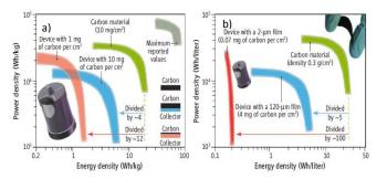
Figure 2. Ragone plots for an electrochemical capacitor. a) Plot based on the gravimetric basis and b) plot based on the volumetric basis. The plots show that excellent properties of carbon materials will not translate to medium- or large scale-devices if thin-film and/or low density electrodes are used. Reprinted with permission.<sup>43</sup>
