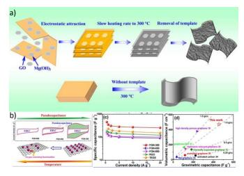
Figure 7. Schematic illustration of the formation of the template-assisted functionalized graphene. Reprinted with permission.<sup>78</sup>
