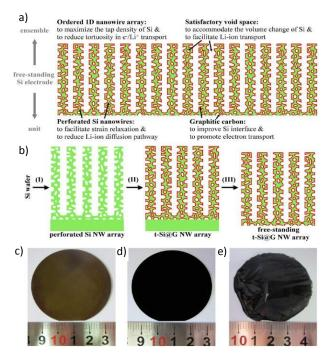
Figure 8. a) Cross-sectional view of a textured silicon@graphitic carbon nanowire (t-Si@G NW) array electrode. b) Schematic of its fabrication process. c), d) and e) Photographs of a perforated silicon nanowire array on a wafer, t-Si@G NW array on a wafer and a free-standing t-Si@G NW array electrode. Reprinted with permission.<sup>95</sup>
