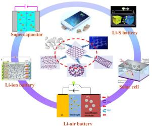
Figure 1. An overview of carbon materials used in EES devices, including lithium-ion batteries, supercapacitors, lithium-sulfur batteries, solar cells and lithium-air batteries.
