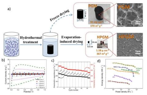
Figure 6. a) Schematic of the self-assembly formation of the highly dense but porous graphenebased monolith (HPGM). b) CV curves of the HPGM at different scan rates. c) Rate performance of HPGM. d) Ragone plot of HPGM compared with other carbon materials. Reprinted with permission.<sup>24</sup>
