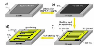
Figure 10. Schematic of the fabrication of a microsupercapacitor integrated onto a silicon chip based on a CDC film. Standard photolithography techniques are used for fabricating a CDC capacitor electrode and the deposition of the gold current collector. Reprinted with permission.<sup>106</sup>
