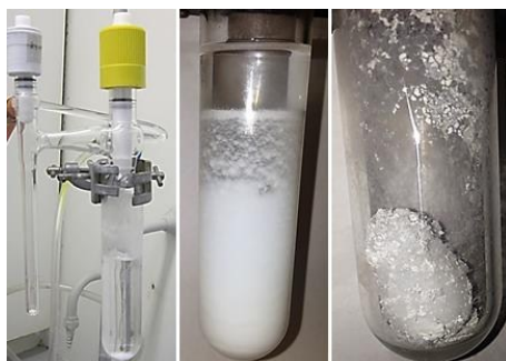
Fig. 2 Images of a typical [\text{NH}_4][\text{OTf}] -catalysed silicon imidonitride preparation immediately after warming to ambient temperature (showing the side-arm used to measure liquid ammonia), after gelation at 24 h aging time, and the xerogel after solvent removal.
