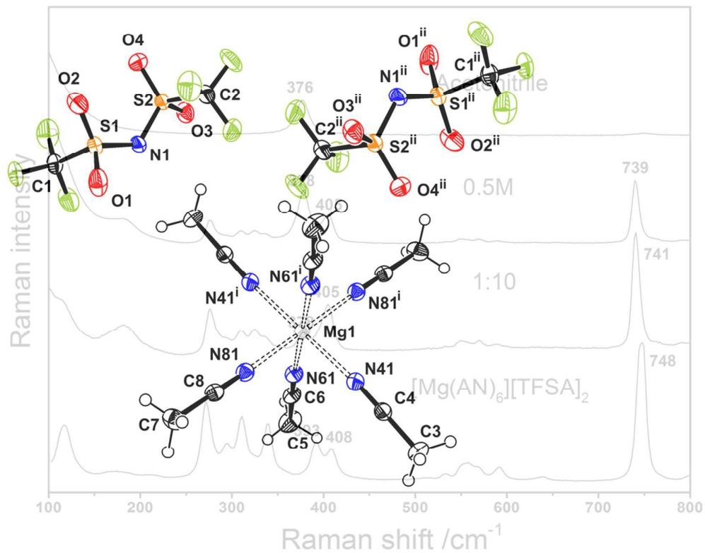
The  $\text{Mg}^{2+}$  ion in the  $\text{Mg}[\text{N}(\text{SO}_2\text{CF}_3)_2]_2\text{-CH}_3\text{CN}$  system is surrounded by six acetonitrile molecules in both the solid and liquid states.
