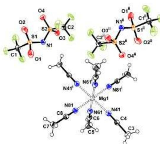
**Fig. 1** ORTEP diagram of the [Mg(AN)<sub>6</sub>][TFSA]<sub>2</sub> complex. Thermal ellipsoids are drawn at 50% probability. Symmetry operations: (i) 1-x, -y, -z; (ii) 1-x, -y, 1-z. Bond length and angles: Mg1...N41 2.1477(12) Å, Mg1...N61 2.1439(12) Å, Mg1...N81 2.1549(12) Å, N41...Mg1...N61 89.11(5)°, N41...Mg1...N81 90.33(4)°, N61...Mg1...N81 89.81(5)°.
