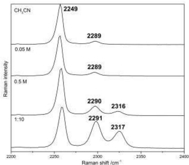
Fig. 3 Raman spectra of pure acetonitrile and acetonitrile solutions of Mg[TFSA]<sub>2</sub> (0.05 M, 0.5 M, and 1:10) between 2200 and 2400 cm<sup>-1</sup>.
