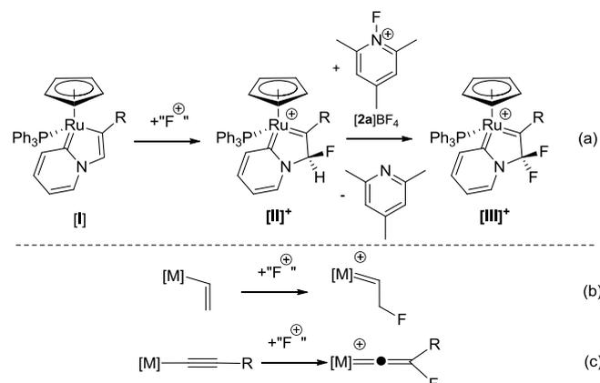
Scheme 1. Outer sphere electrophilic fluorination of an organo-ruthenium complex. "F<sup>+</sup>" = [FTMP]BF<sub>4</sub>, Selectfluor or N-fluorobenzenesulfonimide (NFSI).
