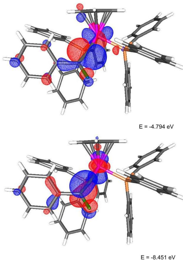
**Figure 1.** LUMO (top) and HOMO (bottom) of **[3a]**<sup>+</sup>
