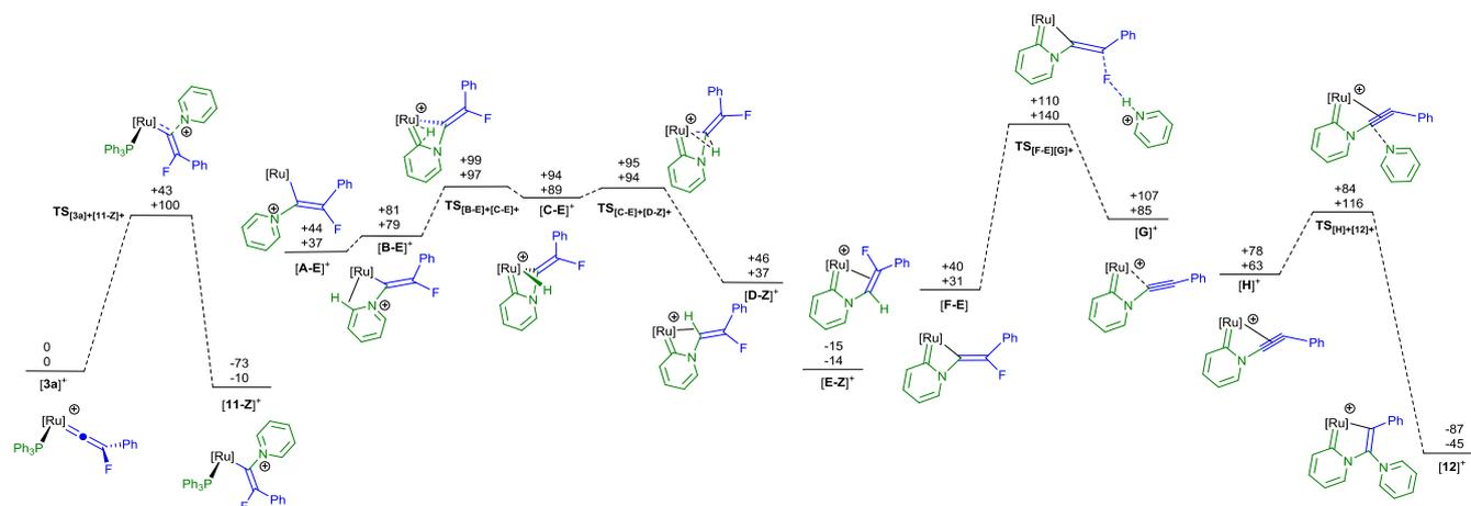
**Figure 5.** Potential energy surface for the proposed mechanism of formation of  $[12]^+$  from  $[3a]^+$ .  $E_{SCF+ZPE}$  (top) and Gibbs energies at 298.15 K (bottom), relative to  $[3a]^+$  and two molecules of pyridine, are shown in  $\text{kJ mol}^{-1}$ . Calculations are at the (RI)-PBE0-D3/def2-TZVPP/(RI)-BP86/SV(P) level with COSMO solvation in pyridine. [Ru] =  $[Ru(\eta^5-C_5H_5)(PPh_3)]$ .
