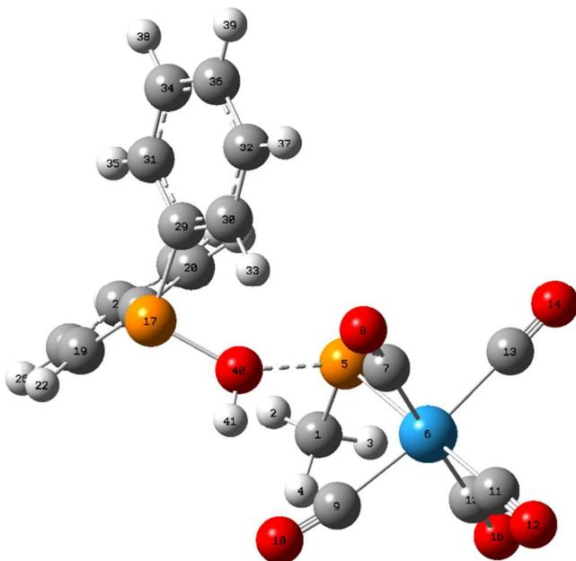
**Fig. 2** Computed structure of the adduct [MeP-W(CO)<sub>5</sub>]-HOPPh<sub>2</sub>. Main bond lengths (Å) and angles (°): P5-O40 2.042, P17-O40 1.770, P5-C1 1.870, O40-H41 0.977; P5-O40-P17 136.06, P5-O40-H41 111.06, P17-O40-H41 109.89, C1-P5-O40-H41 66.96
