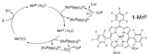
**Scheme 1.** Reaction scheme for the light driven oxidation of an organic substrate by water in the presence of a catalyst/protein conjugate, a Ru chromophore and a Cobalt-based sacrificial electron acceptor. The structure of the applied 1- $\text{Mn}^{\text{III}}$  corrole catalyst is shown on the right. For experimental conditions see experimental section. Protons released during light induced activation of  $\text{H}_2\text{O}$  are omitted for clarity.
