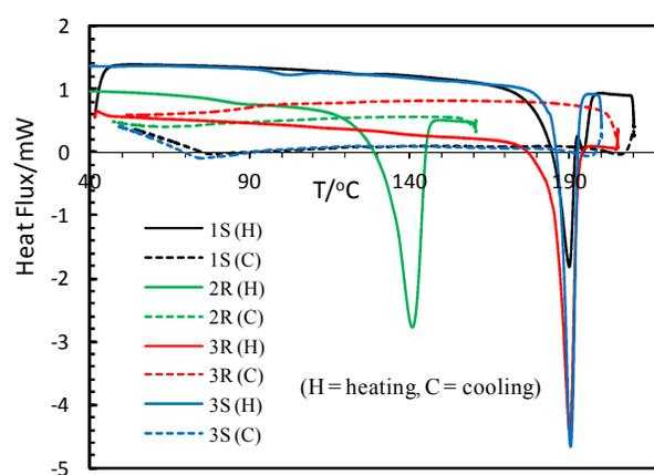
**Figure 6.** DSC analyzes curves of heating and cooling for the compounds.
