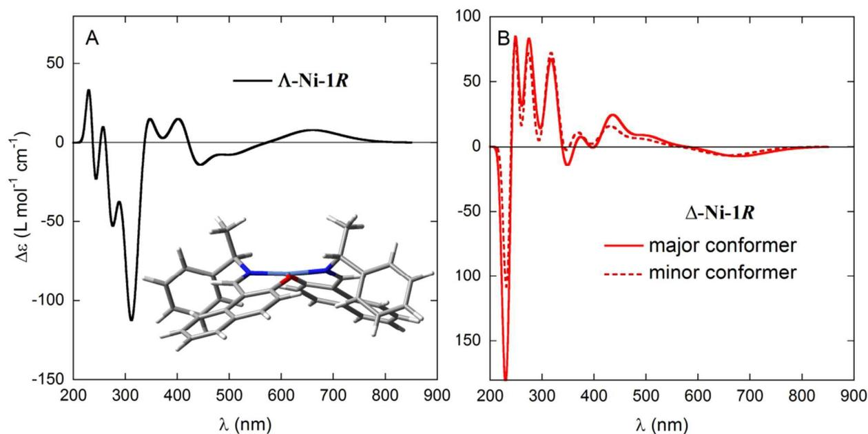
**Figure 2.** CD spectra calculated at the B3LYP/TZVP//B3LYP/6-31G(d) level for the two diastereomers **Δ-Ni-1R** (left, conformation shown in the inset) and **Δ-Ni-1R** (right, two conformations shown in Figure S3). Gaussian band shape with exponential bandwidth  $\sigma = 0.2$  eV.
