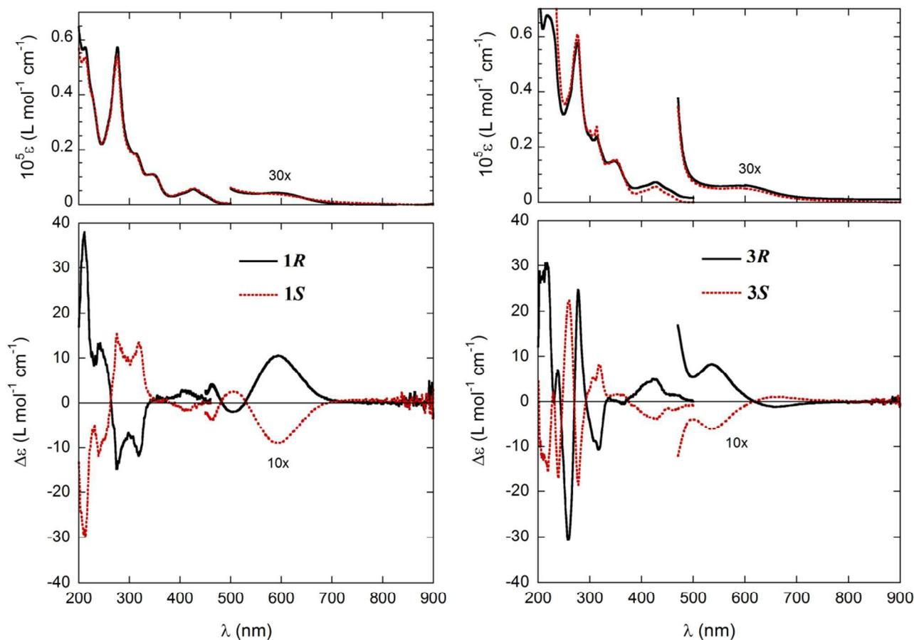
**Figure 1.** UV-vis. and CD spectra of **1R** (0.76 mM), **1S** (0.79 mM) (left), and **3R** (1.95 mM), **3S** (1.96 mM) (right) in cyclohexane; cell path-length: 0.1 mm, 200–500 nm; 5 mm, 425–600 nm; 10 mm, 400–900 nm.
