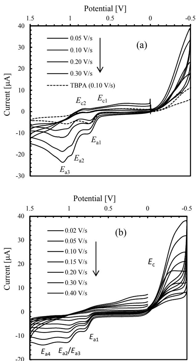
**Figure 7.** Cyclic voltammograms of (a) *S*-HL1 (1.5 mmol/L) and (b) **1S** (1.0 mmol/L); TBAP (0.1 mol/L) at varying scan rates in acetonitrile at 25 °C.
