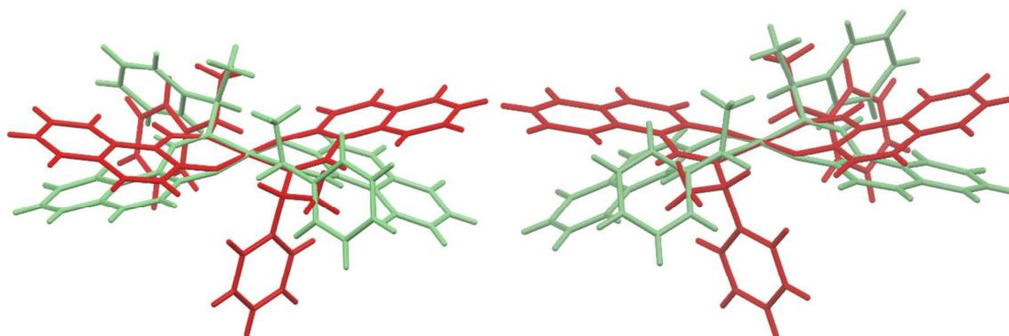
**Figure 4.** Overlay of the two symmetry independent molecules in Ni-R-L1 (**1R**) (left) and Ni-S-L1 (**1S**) (right). The Ni1 molecule **A** is shown in green, the Ni2 molecule **B** in red. The five atoms NiN<sub>2</sub>O<sub>2</sub> were pairwise specified to orient the overlay which was managed with the "Structure overlay" option in Mercury 3.5.1 (copyright CCDC 2001-2014, <http://www.ccdc.cam.ac.uk/mercury/>).
