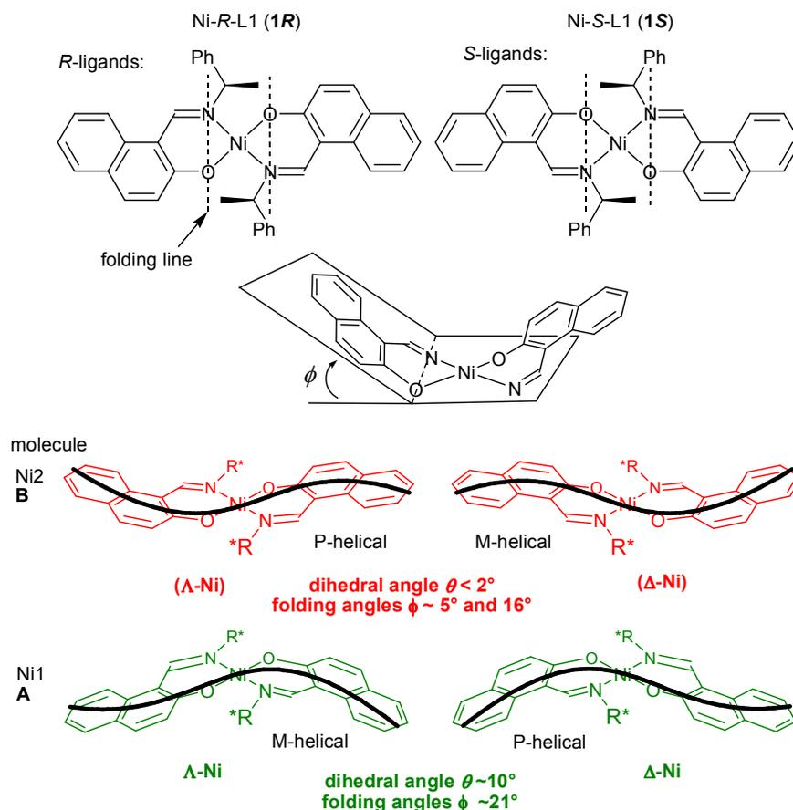
**Scheme 3.** Schematic illustration of the non-planar, skewed *bis*(naphthaldiminato)  $N_2O_2$  ligand arrangement around the nearly square-planar coordinated Ni atom in **1R** (left) and **1S** (right) and definition of the folding angle  $\phi$ . The thick black line depicts the *P*- or *M*-helical arrangement from the envelope conformation in the NiNOC<sub>3</sub> chelate ring together with the curvature in the naphthaldiminato ligand. The round brackets indicated a faint chirality at Ni.
